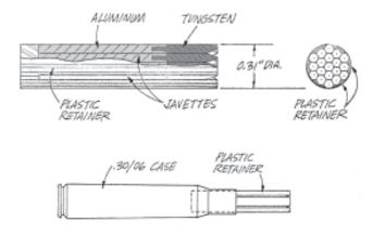
Fig. 28-25. Experimental .30-06 Javette-launching cartridge.
