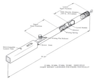
Fig. 28–80. Multi-caliber Gyrojet flare launcher. MBA drawing.
