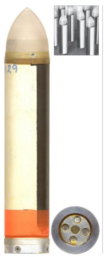
Fig. 28-95. 40mm Type I cloud seeding rocket and MBA photo.
