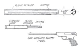
Fig. 28–26. Experimental .25-caliber Javette-launching cartridge.
