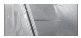
Fig. 28–14. Lancejet perforation of 0.75-inch plywood. MBA photo.
