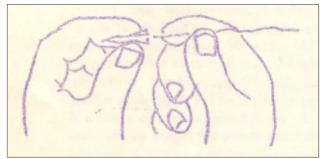
Carefully place the small square of onion skin paper [?] onto the Microjet; press the paper toward the tail so that the fins are halfway inserted. This acts as a hold down, allowing the rocket to build up to full thrust before leaving tube.
